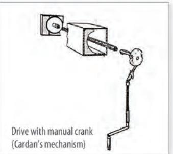
Drive with manual crank (Cardan's mechanism)
